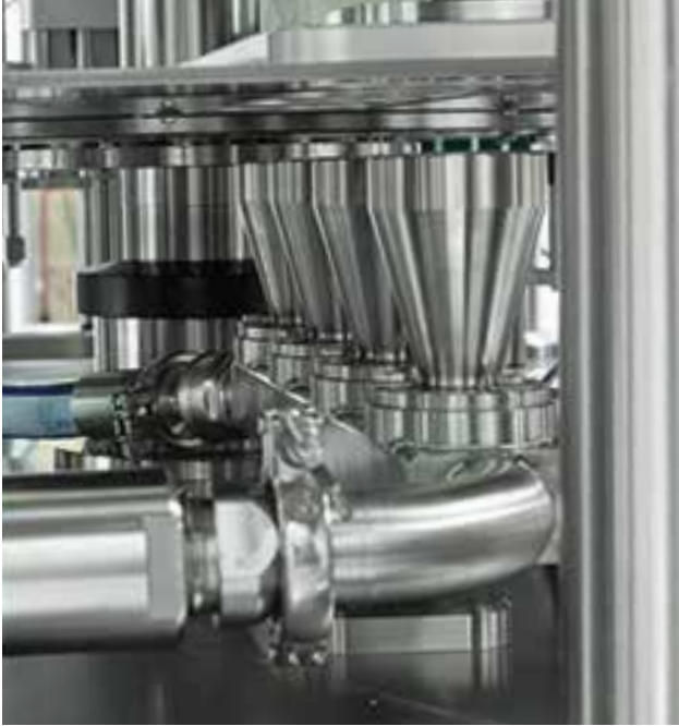
Combined cup lift and CIP manifold.
